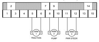
**Section 5.4.3 TMM Pump Control Connections**
